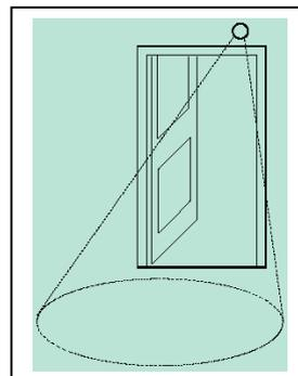
**CDI Services** recommend the use of Abloy active sensors, which provide fast detection, insensitive to colour variations, and are insensitive to reflectivity of ground.
