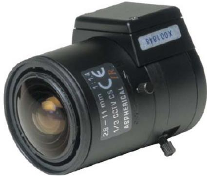
Standard lenses are not optimized for effective 24 hour surveillance as it is often only possible to focus the lens either for daylight operation or night time operation, but not both. However, IR corrected lenses do not suffer from such focussing issues and are able to capture quality images both during the day and under visible, or non visible infra red lighting at night.
